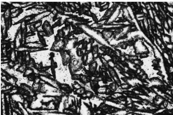
Figure 14 (a) OLM Image of AISI 2507 SDSS tested specimen using optimised DLEPR conditions showing sensitised region
