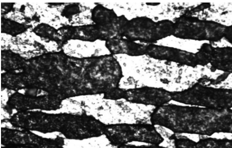
Figure 9 (a) OLM Image of SDSS unsensitised region after conducting DLEPR test using 20% H 2 SO 4 in 0.001 M TA at 70 °C
